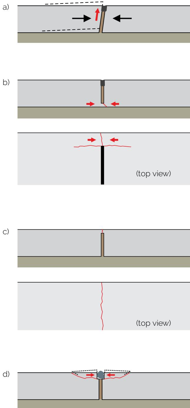
Joint failures due badly positioned filler plates in an expansion joint
