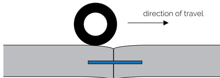
Principle of load transfer between two adjacent slabs
