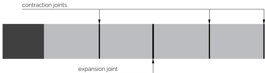
In the case of a concrete-asphalt transition, a "composite joint" is an alternative. It is approximately 250 to 500 mm wide and consists of a mixture of a particular type of bituminous compound and fine gravel. The capacity of such a compound seal is 10 or even 15 mm in expansion and contraction.
