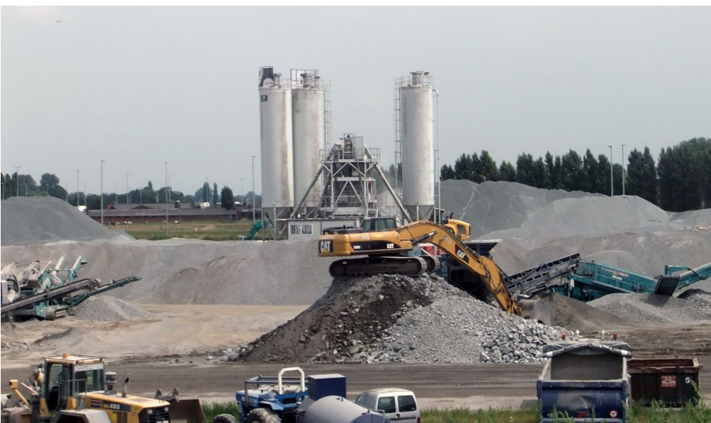
Recycling of crushed concrete aggregates as part of a local and circular economy - Photo: Luc Rens
