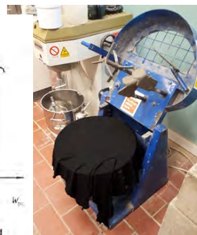
Figure 1 — Determination of W_{pc} by compacting method
