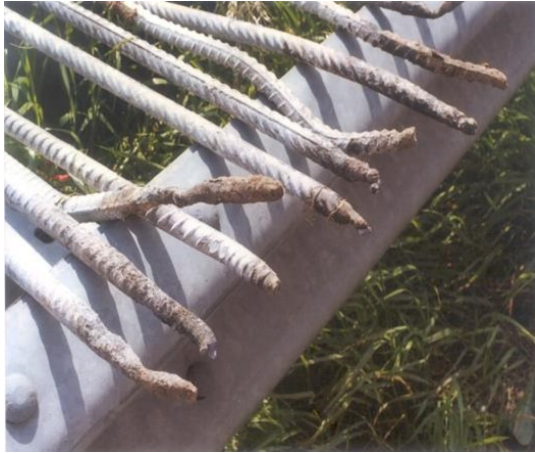
Corroded reinforcement bars at transverse construction joint in CRCP
