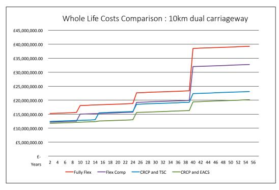
At 40 years, the Fully Flexible Pavement option will be almost 2.5 times more expensive than the Exposed Aggregate Concrete Surface.
