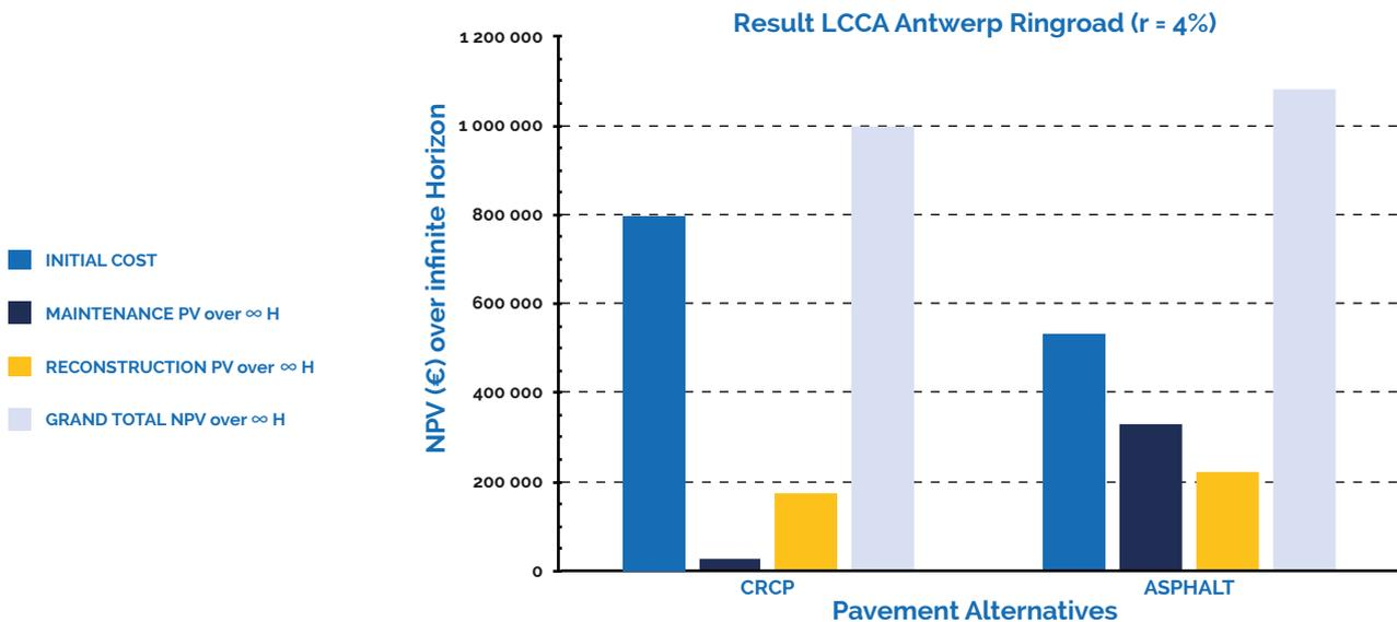
Although the initial cost of the concrete alternative is 50% higher than that of the asphalt alternative, both alternatives have nearly the same net present value over an infinite horizon for a real discount rate of 4%. This is clearly due to the fact that the asphalt alternative requires a substantially higher present investment to pay for future maintenance and reconstruction.
