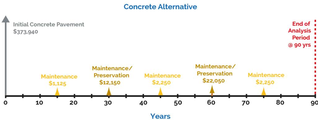
Table 5-5. Concrete Alternative – NPV Calculation (r=3%)
