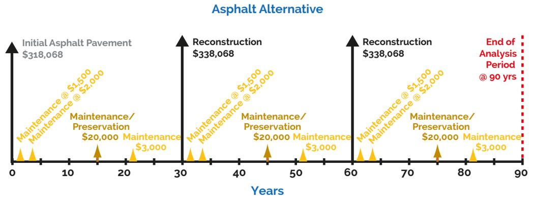
Table 5-6. Asphalt Alternative – NPV Calculation (r=3%)
