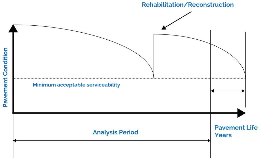
Figure 3-1 shows a typical analysis period for a pavement design alternative. Note that the curve in this figure is a simplified theoretical representation that is commonly used in LCCA publications to depict
