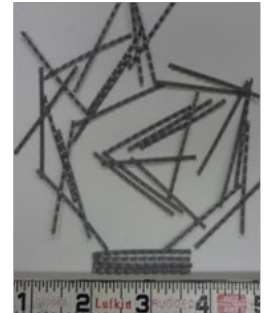
Crimped synthetic: Enduro 600
