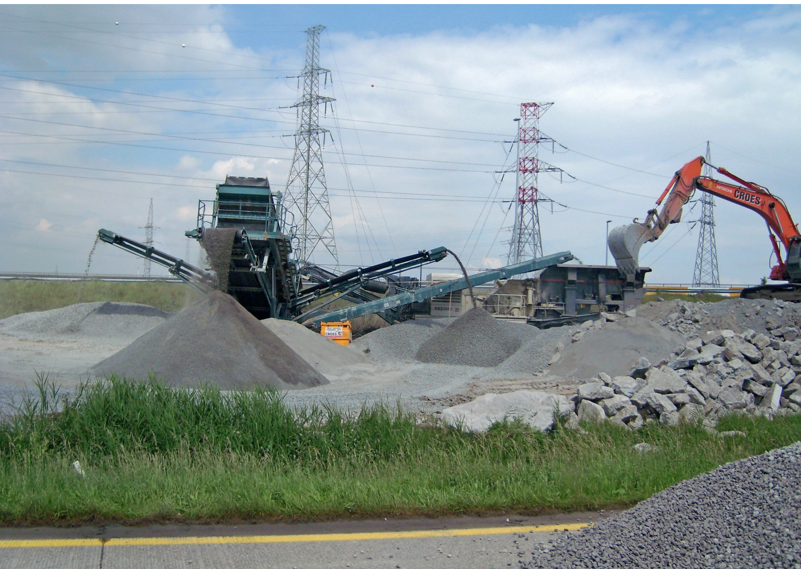
Crushing and sieving installation at motorway N49, Zwijndrecht, Belgium, 2007 © AWV, Flemish Agency for Roads and Traffic
