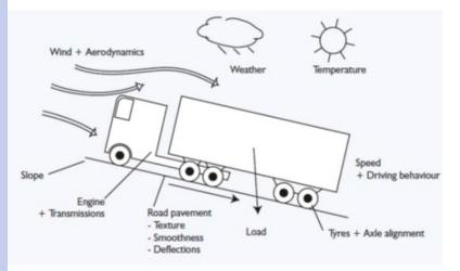
Evenness and texture depend on the quality of construction and/or safety requirements, both for concrete and asphalt roads. This includes the absence of undulations, uneven patches, rutting, potholes or deteriorated joints.
