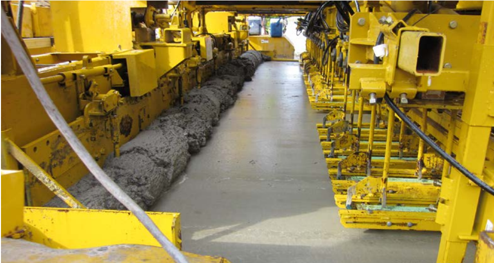
Dowel bar inserters (Wirtgen – Gomaco – G&Z)
