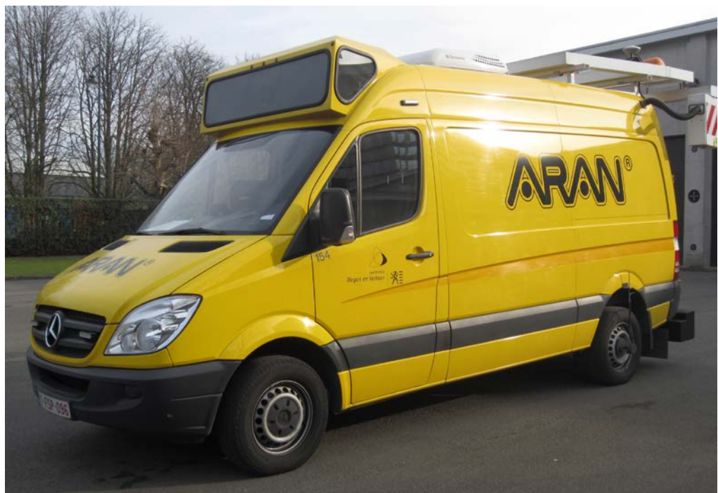
ARAN (Automatic Road Analyzer) equipped with a laser system to measure transverse profiles
