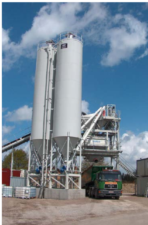
Mobile concrete batching plant
