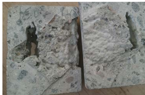
Inadequate compaction of concrete on top of the inserted dowel, leading to voids in the pavement
