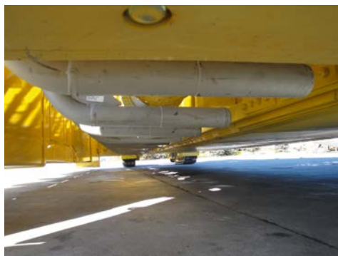
Close-up at the vibrators of a slipform paver
