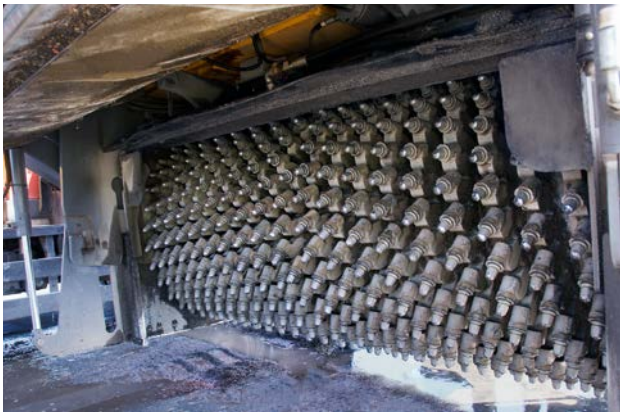
Machine for fine milling and milling drum
