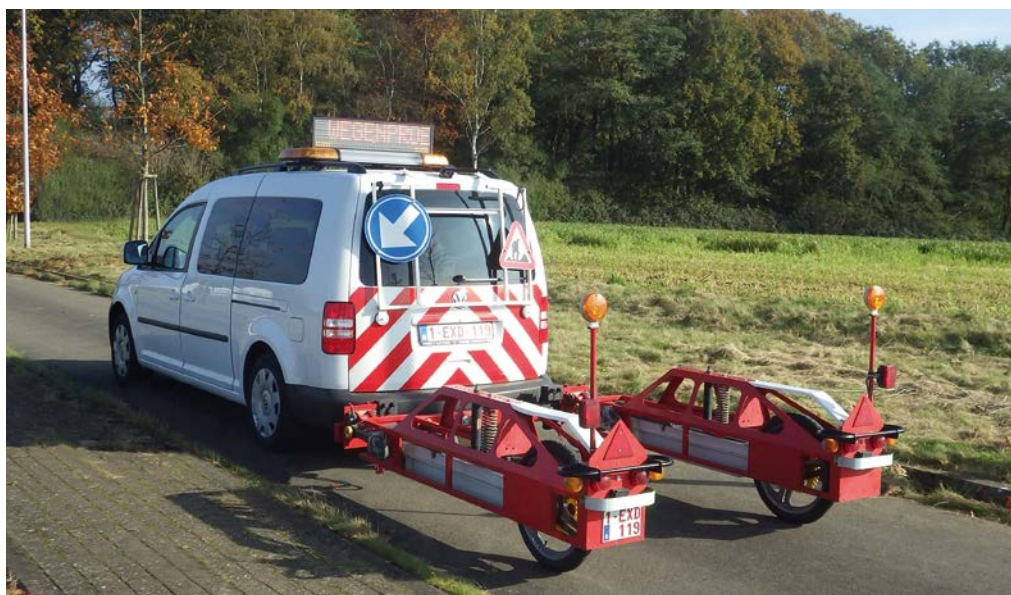
Measurement devices for longitudinal evenness: the APL profiler ("Analyseur de Profil en Long") and a light profiler for bicycle paths
