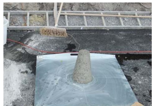
Slump test on site to check constancy of workability
