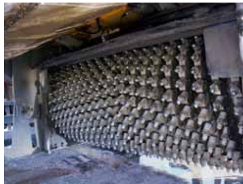
Detail of the milling drum and fine milling machine in operation Photos: Wirtgen
