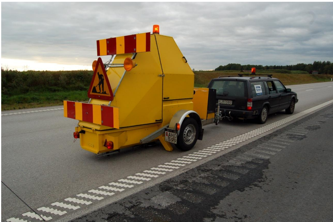
Figure 1. The FWD at the PCC test site on highway E4.
